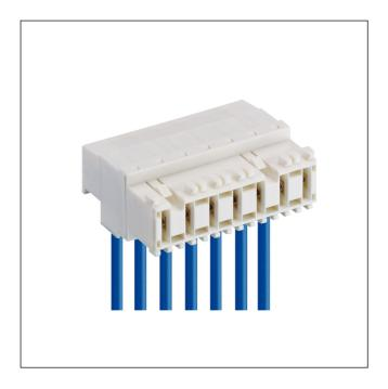
RAST 5 connector for indirect mating, with screw terminal, with lift clamp with protection against misplacing, with test holes and interior locking, consecutive placement without loss of pitch, cable departure opposite to lock
