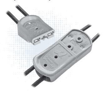
SBS® Mini Connector series is our smallest DC power connector in the SB® group. The SBS® Mini securely holds two crimp and poke contacts with sacrificial tips to enable hot swap capabilities on DC circuits. The low resistance contacts accept 20 to 10 AWG (0.75 to 4.0 mm²) wires allowing up to 52 amps of UL rated performance per position.
